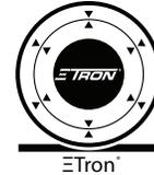
**ETRON®** is a technology developed by Shunyata Research that prevents dielectric absorption and re-radiation in signal transmission. It requires a special type of conductor that has two signal paths and an electric field compensation circuit that creates a cancellation signal that prevents the insulation from developing a charge. **ETRON®** cables preserve the integrity of the source signal even when using very long runs of cable.
