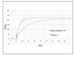
This graph demonstrates the profound effect that a purposefully crafted wire geometry can have on DTCD<sup>™</sup> versus a conventional wire geometry in a more standardized design.
