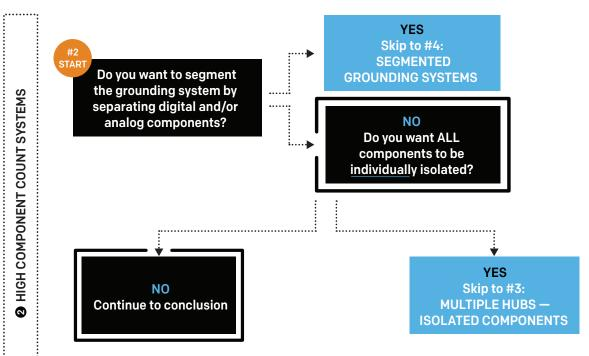
**CONCLUSION:** You have more than 6 components that need to be grounded but you DO NOT want the expense and complexity of multiple hubs. If this is correct, we recommend: **1** ALTAIRA: Chassis Model (CG-NR)
